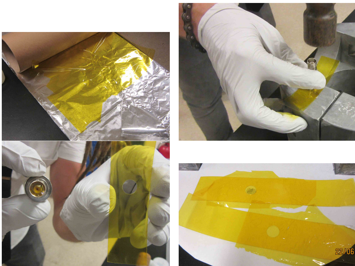
Fig. 21 Punching the kapton tape and attaching 8 \mu\text{m} kapton film to the double-side kapton tape.
