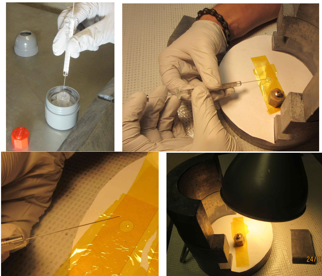
Fig. 23 Dropping ^{22}\text{NaCl} aqueous solution on the Kapton film.
